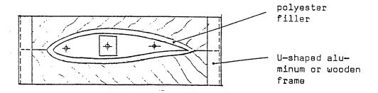
U-shaped aluminum or wooden frames make the positioning of the templates easier when bonding the winglet connection in place. Be sure to apply sufficient parting agent to templates to avoid any bonding.
