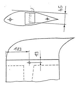
Next trim the root rib(s), cover with tape or a similar parting foil and apply a parting agent, then insert the GFRP wing tip connecting rib (included in the kit) into the wing and fit the wing tip, previously cut off, to rib and wing — any remains of spar and shear web can be removed. With all components brought to proper shape and their mating surfaces sanded, bond wing tip to its connecting rib, secure in proper position and attach the two—piece templates.
